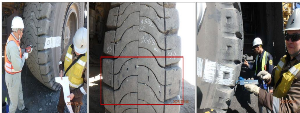
Figure 3: During the investigation of the internal thermal condition of ultra-large tires.
