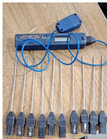
Figure 2: Needle-type thermocouple (TA410-2) and TASCO TNA-20 digital thermometer used in the experimental tests.
