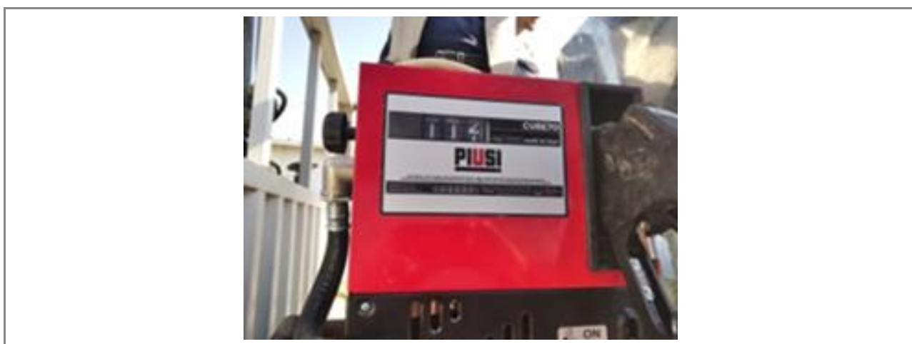
Figure 5. PIUSI digital fuel-flow meter used for registering fuel consumption during GTL field testing.
