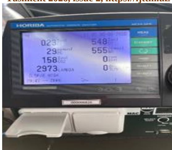
Figure 7. HORIBA gas-analysis display used to record exhaust-gas parameters during experimental evaluation.
