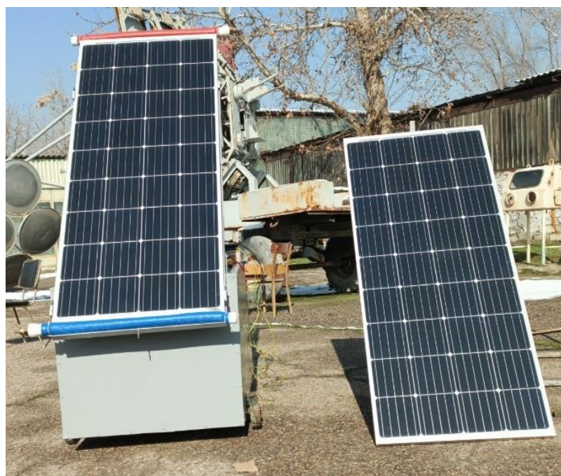
Fig 1. Front view of PVTs with heat collectors made of cellular polycarbonate and polyethylene soft tubing.
